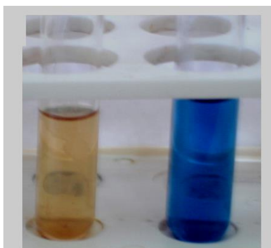
Photo Plate 2: Liquid CAS Assay for Siderophore Production A) Test B) Control
